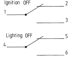
Notes. The double pole switch is suitable for a cdi system which requires the ignition to be earthed to stop the engine.
