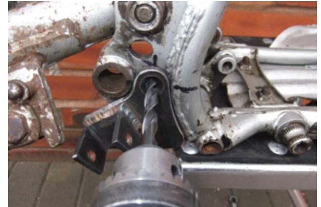
8. RH side - Using footrest bracket as a template drill a second 8mm hole as shown
