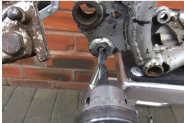
7. RH side - Drill an 8mm hole and insert the supplied bolt from the rear of the hole to secure footrest bracket
